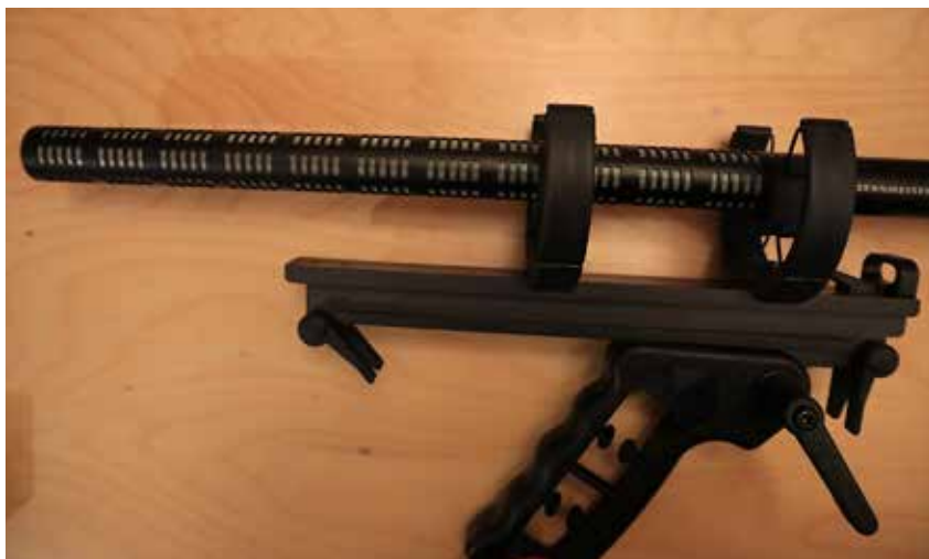
Image 3. Shotgun microphones with interference tube. Photo: Sunny Tseng
