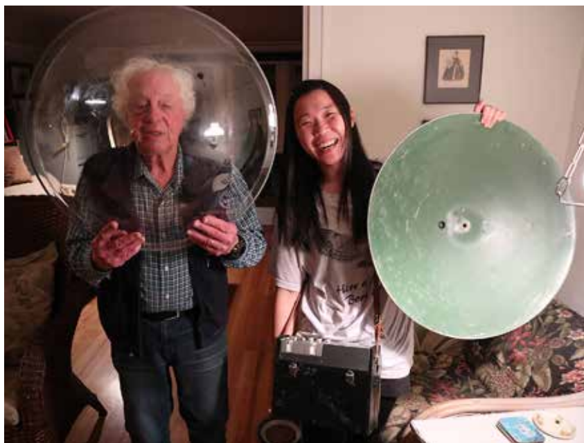
Image 2. The dish can be made of various materials. The most advanced disk is made of foldable plastic which is light and easier to carry in the field (the disk on the left held by Ken Hall). An older version of the dish was made of glass fibre (the disk on the right held by Sunny Tseng). Photo: Peter Ward
