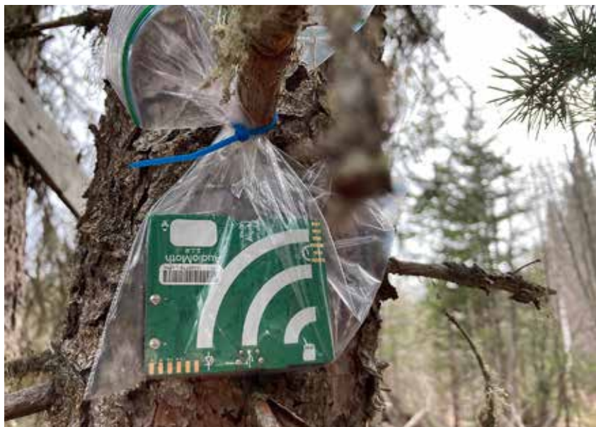
Image 4. Autonomous recording unit AudioMoth. A single autonomous unit includes microphone and data logger that can be left in the field for days or months. Usually, the AudioMoth is deployed with plastic bags to prevent water damage. Photo: Sunny Tseng
